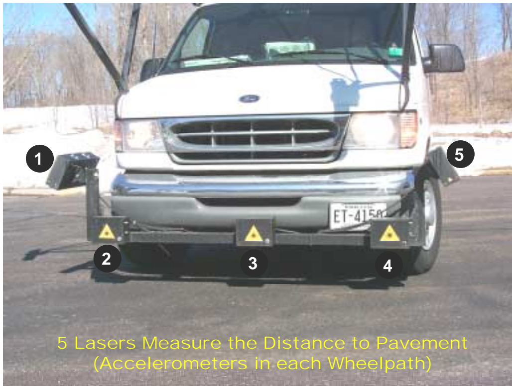
Figure 2. Close-up of lasers used to measure roughness, rutting & faulting.
