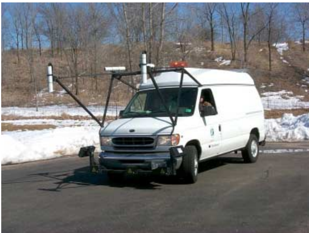
Figure 1. Mn/DOT's Pathway Services, Inc. Video Inspection Vehicle (VIV)
