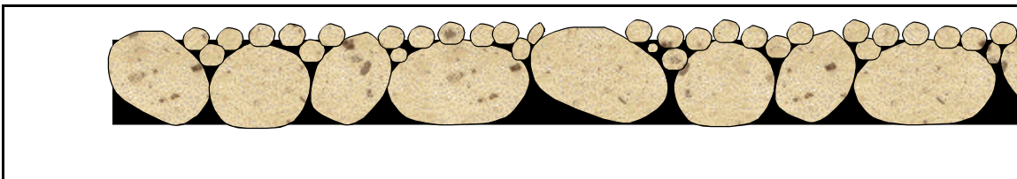
Figure 8.9. Schematic of a Choke Seal (One layer of binder two layers of aggregate)
