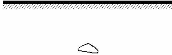
Figure 7. Sketch of object that represents (a) void (Figure 8a) or (b) obstacle (Figure 8b).
