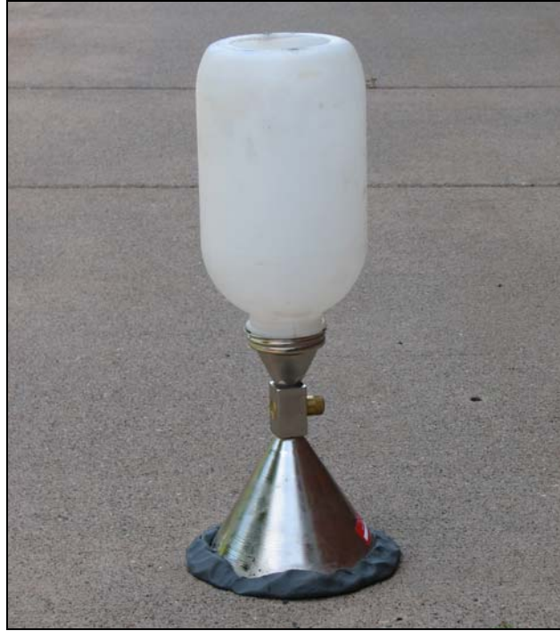
FIGURE 3 In-situ hydraulic conductivity measurement device.
